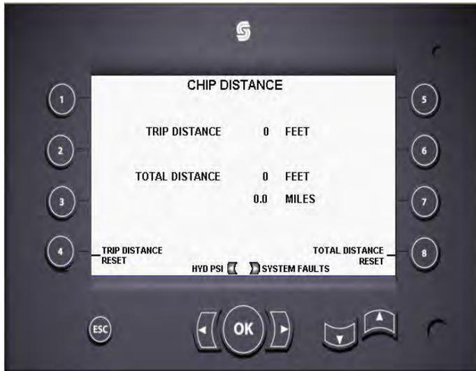
This screen displays the distance traveled while chip spreading. Totals will only advance when the gate is open.
