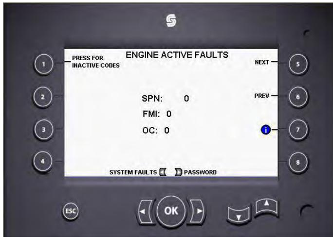
This screen will display any engine faults codes received from the engine controller. Button 5 and 6 are used to scroll through the fault codes.
