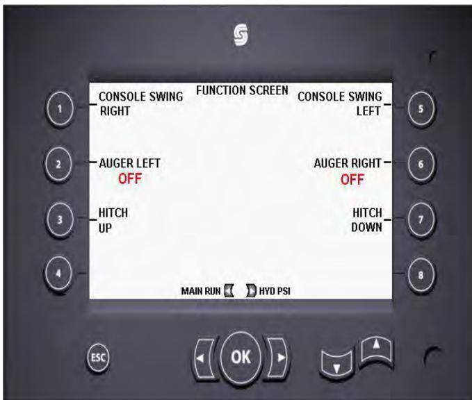
This screen has controls various options for the Console Swing, Augers (not available with CCH Hopper) and Hitch Up/Down.
