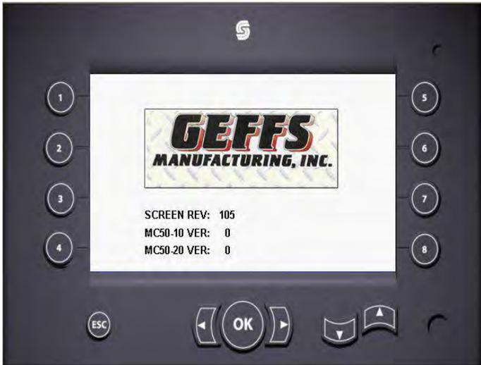
This screen is displayed at power up and shows the current revision level of the installed Plus+1 software.
