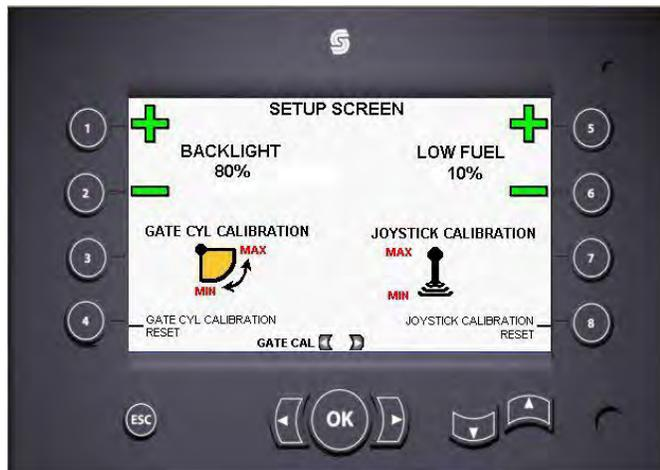
This screen is for setting brightness, low fuel level, Joystick and Gate cylinder input calibration.
