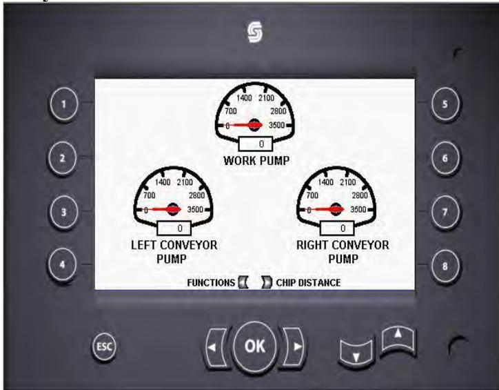
This screen displays the hydraulic pressure of the Work, Left Conveyor and Right Conveyor pumps.
